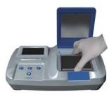
Switch On the eStain<sup>®</sup> 2.0 Protein Staining Device. Press and hold Min. button for 2 seconds to shift to numbering mode. When the upper three digits are flashing, press Reset button to zero.
