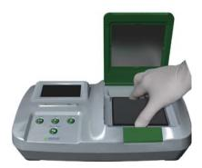
Tear the sealing of a new Graphite Electrode package and take the new Graphite Electrode out of the package. Place the new Graphite Electrode into the anode tank and close the lid of the device.
